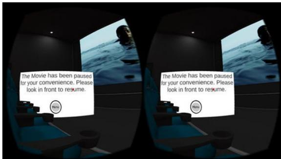
Fig. 2. When the user the stops viewing the screen, the movie is paused and as soon as he is watching it again , the movie is resumed and the pause hovering card goes away. This card can also be used to open the “remote control menu”
