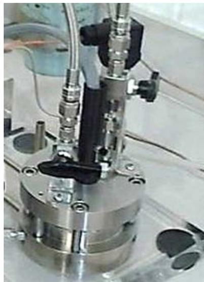
*Figure 4--High Pressure OTR Prototype. Top of chamber shows (left to right) Nitrogen Inlet Valve, Oxysense Analyzer light pen, Chamber Isolation Valve.*
