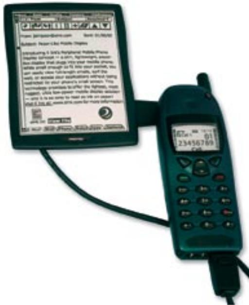
Figure 10. This add-on display is what E Ink calls a "peripheral monitor." Its purpose is to enable mobile phone users to have small handsets while also having the capability to display high-information content when necessary. (Photo courtesy of E Ink, ©2003)
