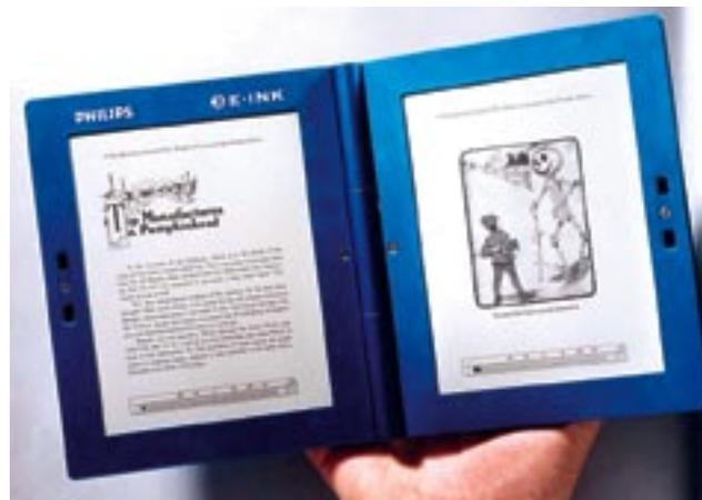
Figure 6. This prototype double-page e-reader, combining an E Ink display and Philips TFT backplane, is the first commercial product resulting from the E Ink and Philips partnership. (Photo courtesy of Philips. Used with permission.)
