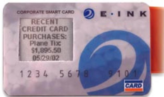
Figure 8. E Ink Corporation has introduced the world's thinnest active matrix display—just 0.3 mm thick, or half the thickness of a credit card. The company is working with leading device makers to integrate these ultra-thin electronic ink displays into next generation portable devices by 2004-2005. (Photo courtesy of E Ink, ©2003)
