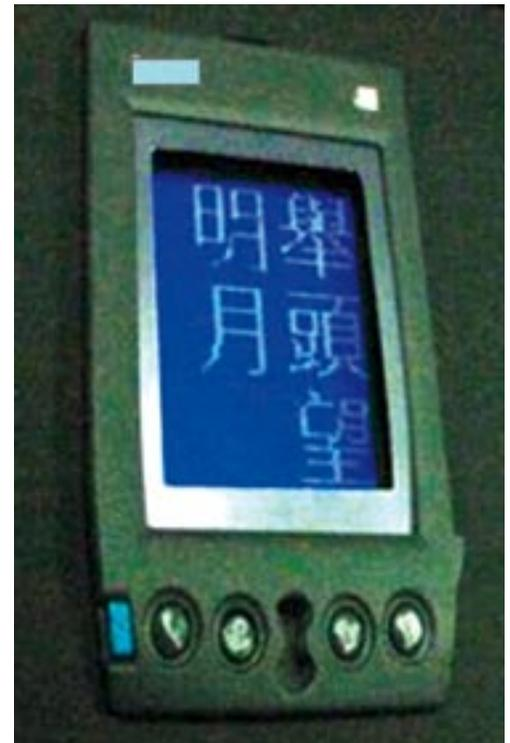
Figure 20. A personal digital assistant (PDA) prototype utilizing the Microcup display technology. (Photo courtesy of SiPix)
