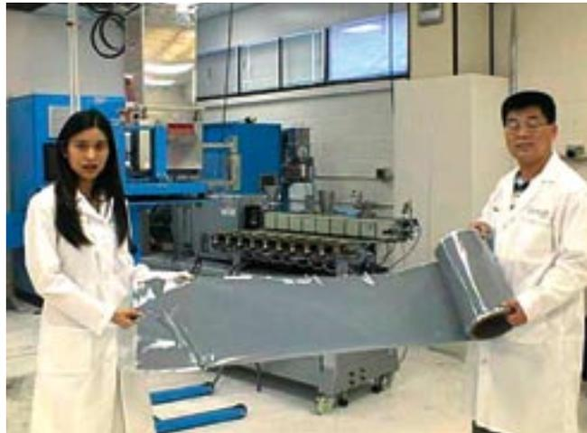
Figure 14. The Gyricon Bead Machine, in the background, produces the 90  $\mu\text{m}$  (micron) beads that form the active layer of the Gyricon media material. Pictured here are Martin Lu, director of Research and Development, and Kailin Chen, engineer. The company was spun off from Xerox Palo Alto Research Center (PARC) in 2000, although the company still has research labs in that facility. (Photo courtesy of Gyricon Media)
