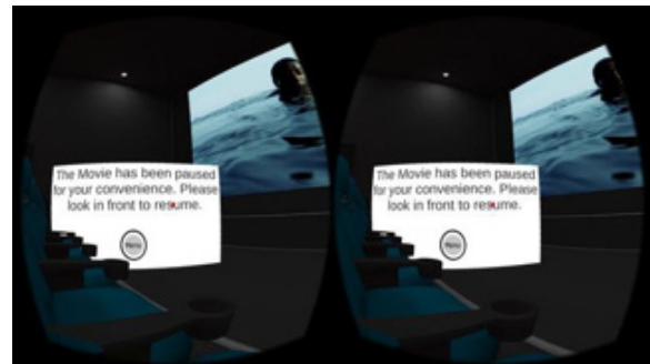
Figure 2 - When the user stops viewing the screen, the movie is paused and as soon as he begins watching it again, the movie is resumed and the pause hovering card goes away. This card can also be used to open the "remote control menu"
