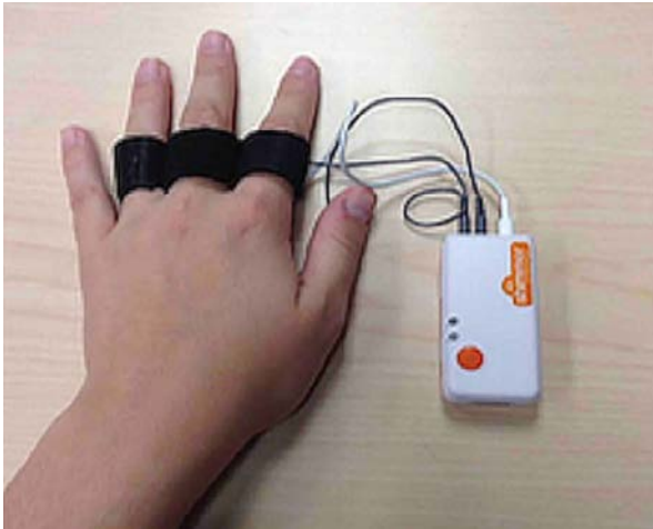
Fig. 2. Shimmer3 device used to capture and record GSR signals from subjects.
