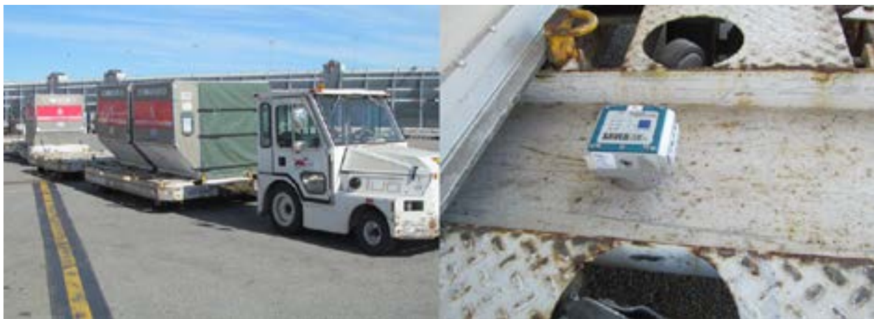
Figure 4: Instrumentation of dollies with SAVER 3X90® data Loggers
