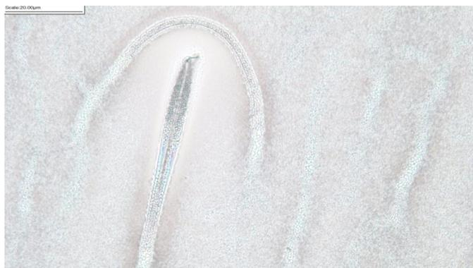
Fig. 2. PS-b-PDMS on HMDS treated wafer de-wetting at 10x magnification
