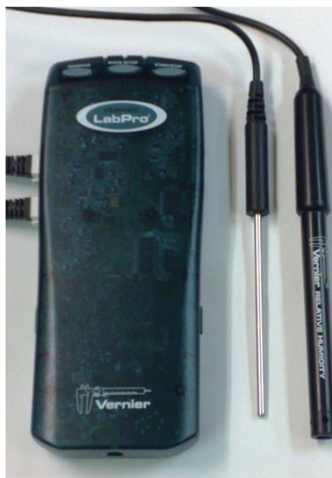
Figure 1: Vernier LabPro with probes
