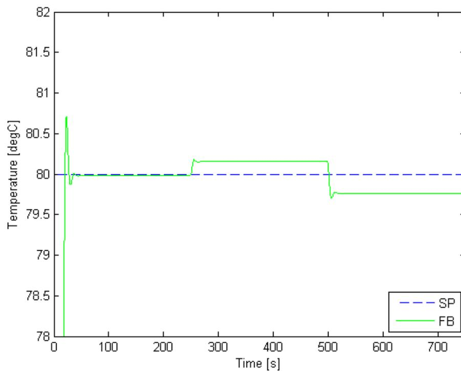
Figure 3-15 Stack Outlet Temperature: 0.6 A/cm<sup>2</sup>: State Feedback Control
