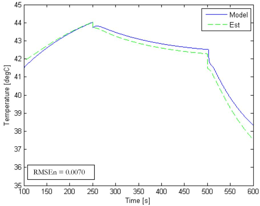
Figure 3-32 State 2: Radiator Wall Temperature, 0.2 A/cm2
