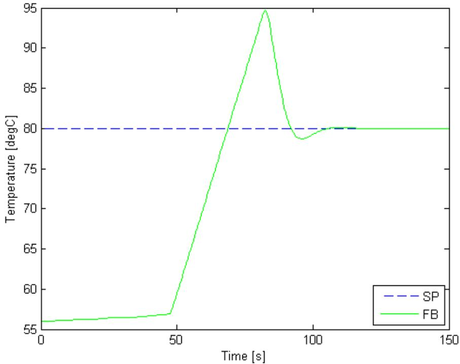
Figure 3-7 Coolant Outlet Temperature during Start-up Conditions
