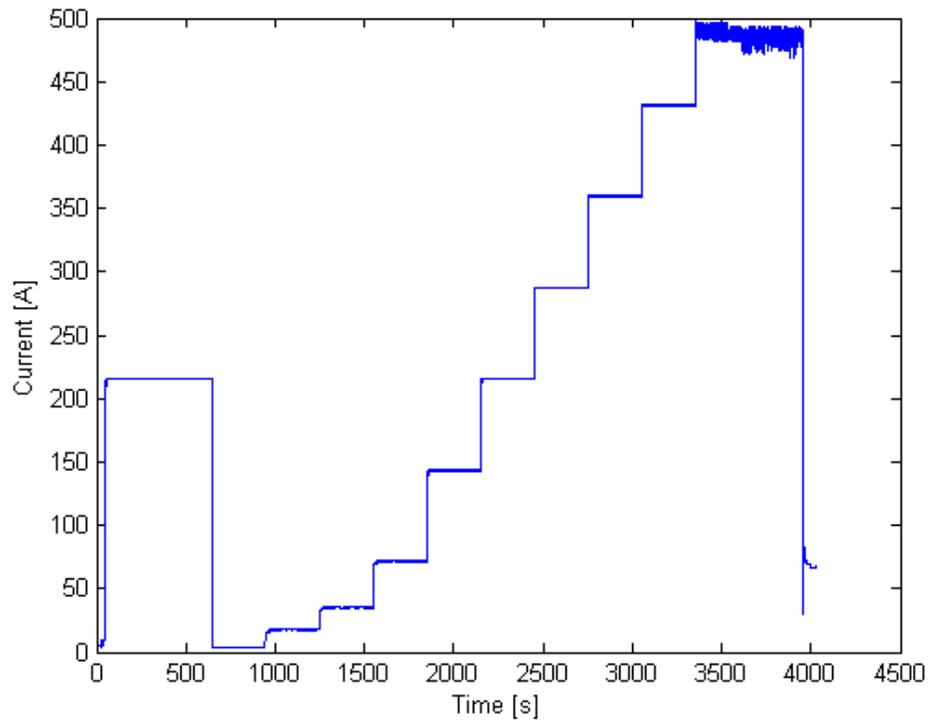
Figure 2-15 Model Validation Pol Curve Current Profile
