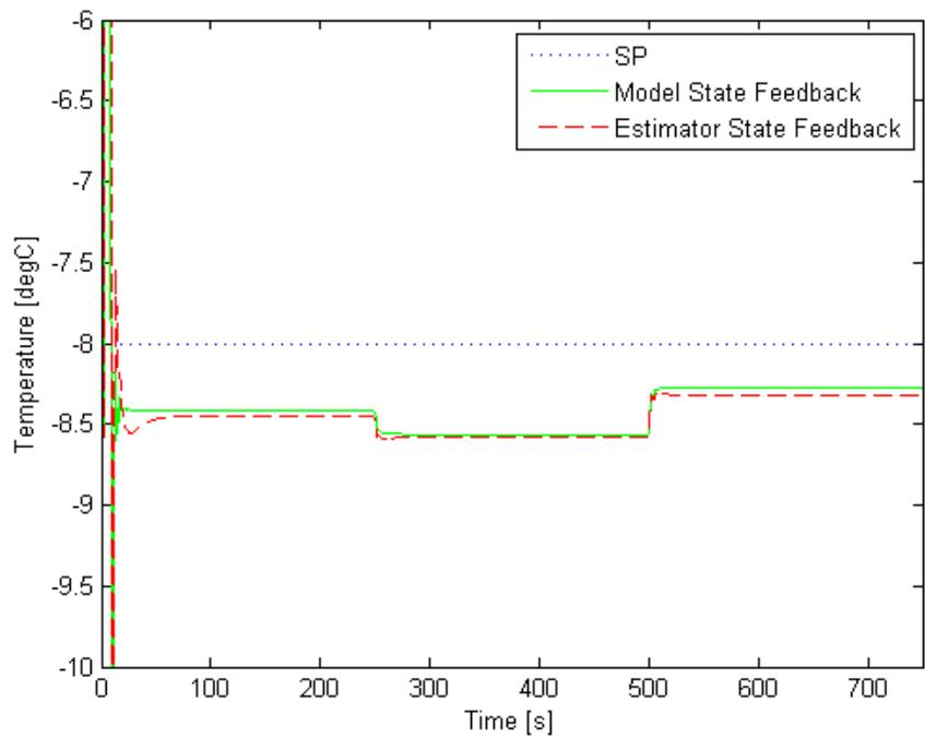
Figure 3-46 Stack Coolant  $\Delta T$ : LQR Control with and without Estimator, 1.2 A/cm<sup>2</sup>
