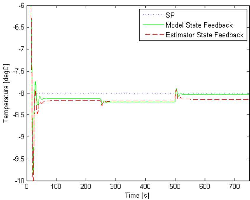
Figure 3-44 Stack Coolant  $\Delta T$ : LQR Control with and without Estimator, 0.6 A/cm<sup>2</sup>
