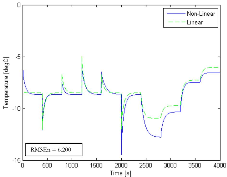
Figure 2-37 Stack Coolant delta T at 0.6 A/cm<sup>2</sup>
