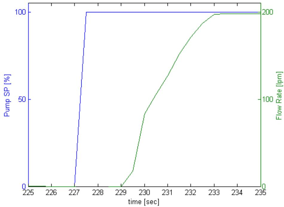
Figure 2-10 Pump Step Response
