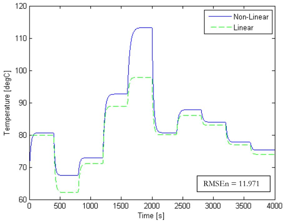
Figure 2-39 Stack Coolant Outlet Temperature at 1.2 A/cm<sup>2</sup>
