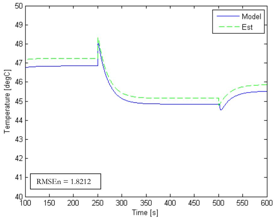
Figure 3-37 State 1: Radiator Coolant Outlet Temperature, 1.2 A/cm<sup>2</sup>
