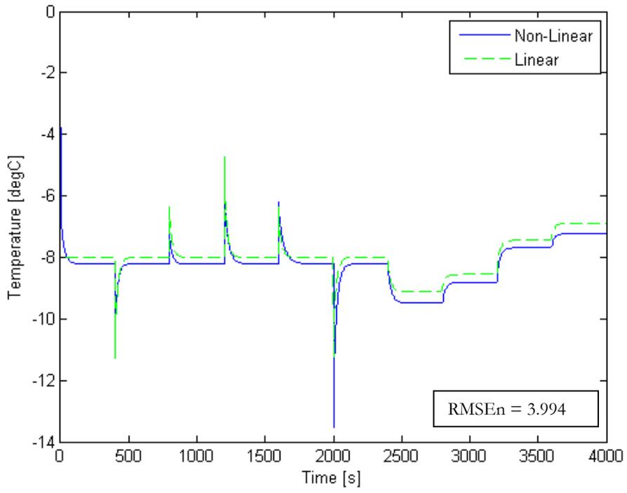
Figure 2-40 Stack Coolant delta T at 1.2 A/cm<sup>2</sup>
