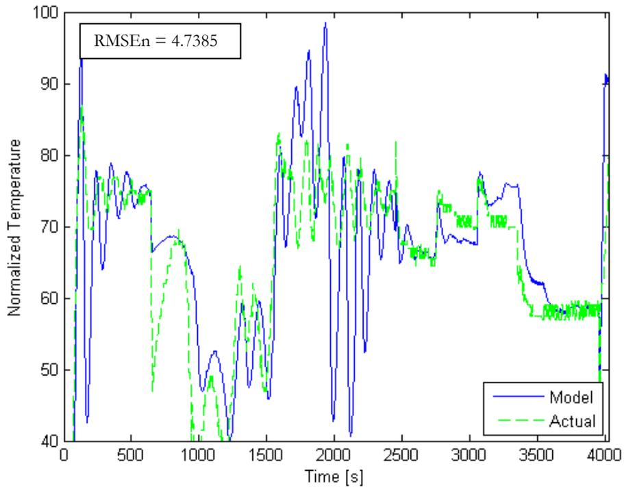
Figure 2-17 Model Validation: Stack Outlet Temperature
