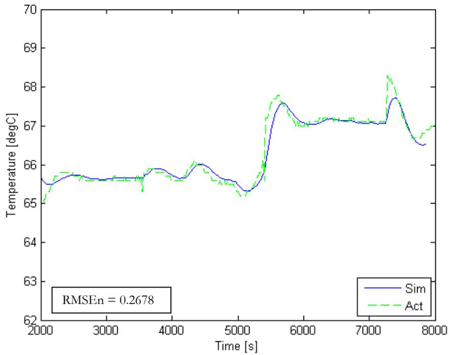
Figure 2-8 Simulated and Actual Stack Coolant Outlet Temperature, Transient
