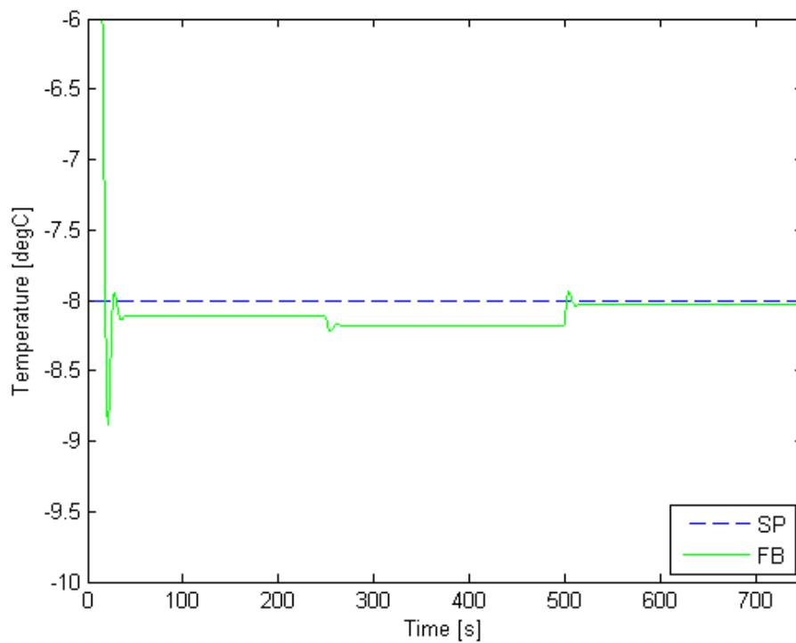
Figure 3-16 Stack  $\Delta T$ : 0.6 A/cm<sup>2</sup>: State Feedback Control
