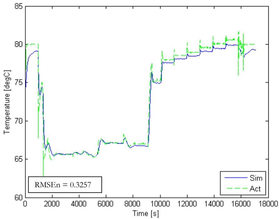
Figure 2-7 Simulated and Actual Stack Coolant Outlet Temperature
