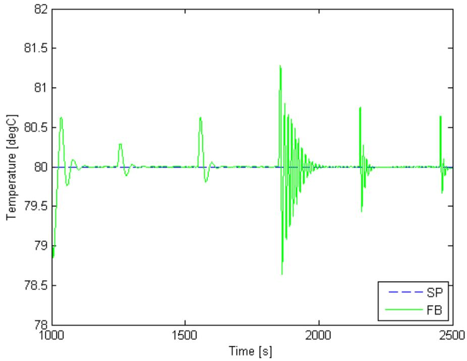
Figure 3-9 Stack Coolant Outlet Temperature: Independent PI Control
