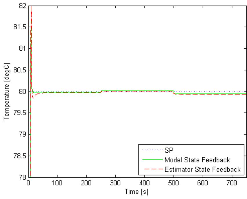
Figure 3-45 Stack Coolant Outlet Temperature: LQR Control with and without Estimator, 1.2 A/cm<sup>2</sup>
