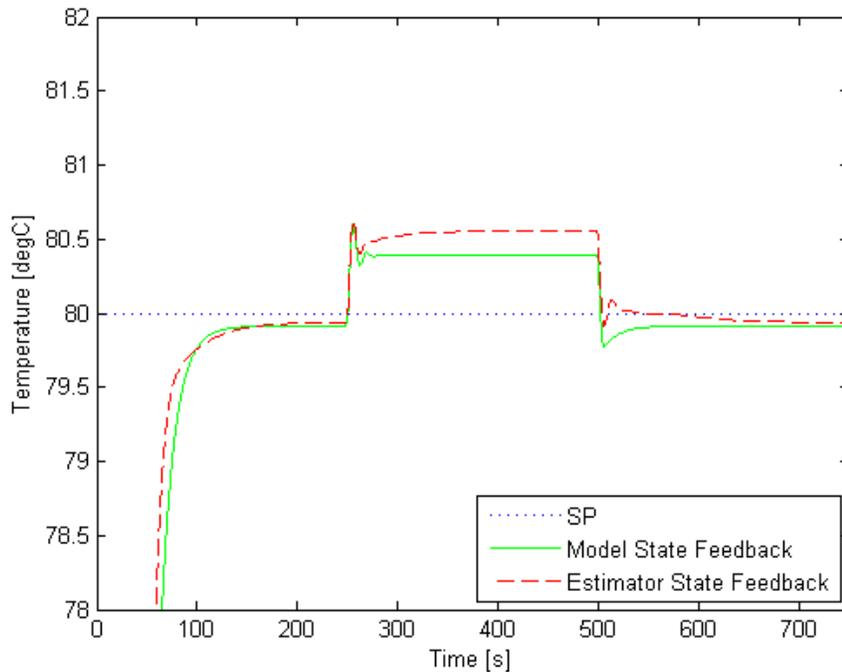
Figure 3-40 Stack Coolant Outlet Temperature: LQR Control with and without Estimator,  $0.2 \text{ A/cm}^2$
