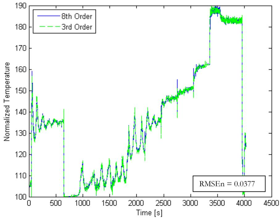
Figure 2-28 Stack Coolant  $\Delta T$  Comparison
