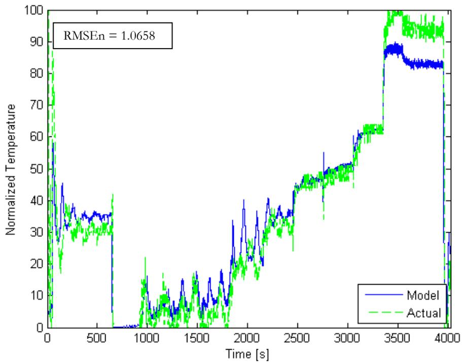
Figure 2-18 Model Validation: Stack  $\Delta T$
