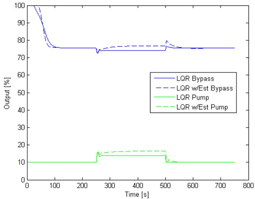
Figure 3-42 Control Effort: LQR Control with and without Estimator,  $0.2 \Delta/cm^2$
