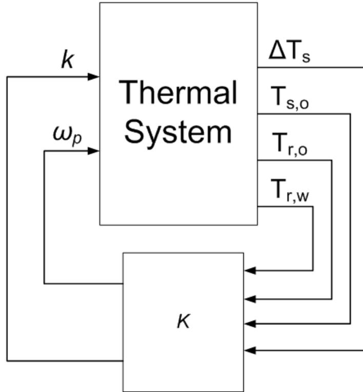
Figure 3-19 Augmented LQR Control with Output Feedback
