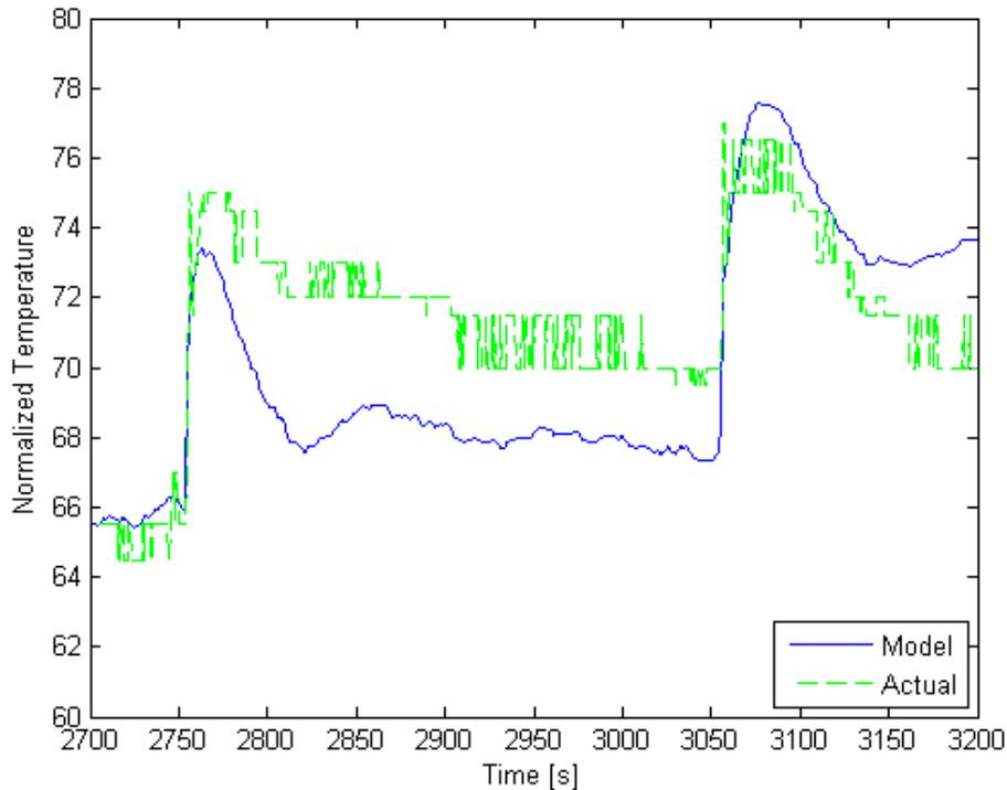
Figure 2-20 Model Validation: Stack Outlet Temperature Transient Response
