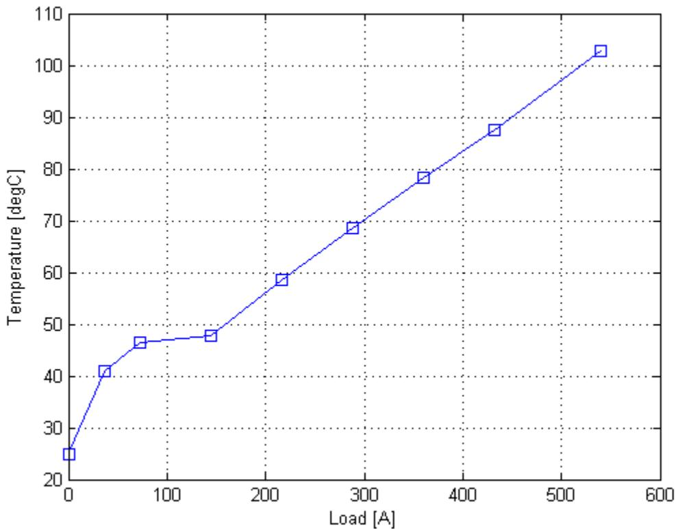
Figure 2-12 Compressor Outlet Temperature as a Function of Load
