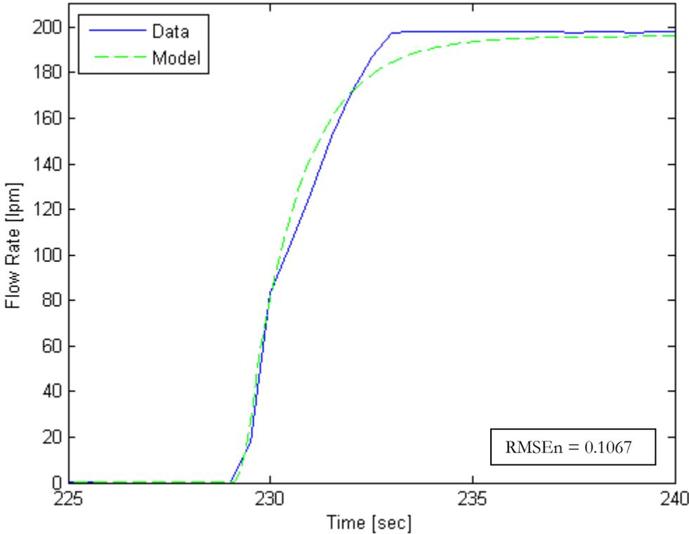
Figure 2-11 Coolant Pump Model Comparison
