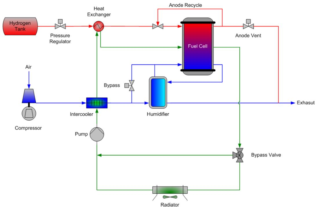
Figure 2-1 Typical Automotive Fuel Cell System Mechanization
