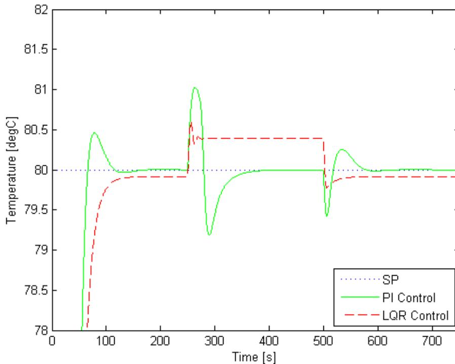
Figure 3-29 Stack Outlet Temperature: Revised PI Tuning
