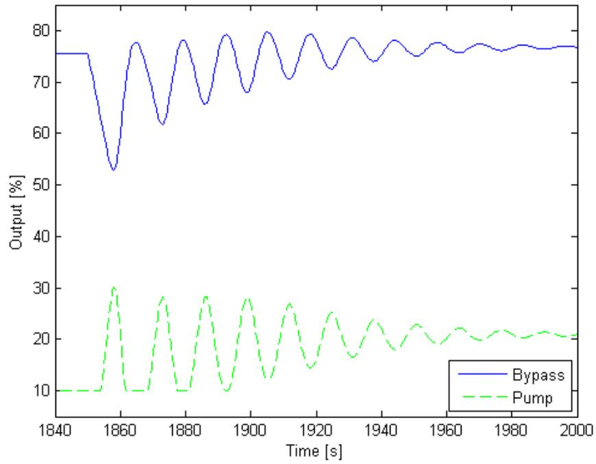
Figure 3-12 Controller Response for Step Change in Current from 0.2 A/cm<sup>2</sup> to 0.4 A/cm<sup>2</sup>: Independent PI Control
