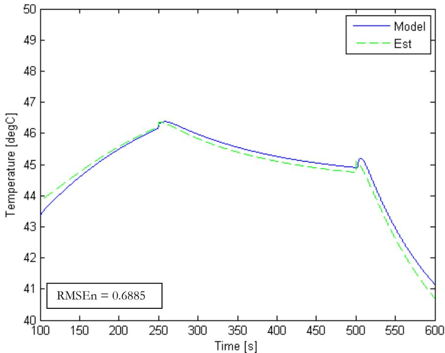
Figure 3-31 State 1: Radiator Coolant Outlet Temperature, 0.2 A/cm<sup>2</sup>
