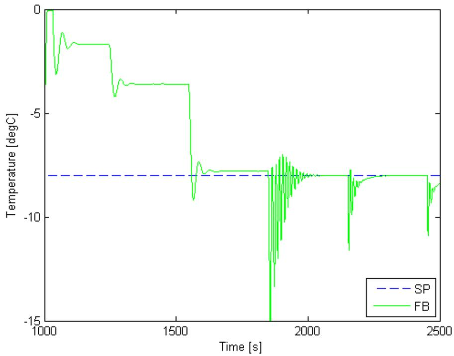
Figure 3-10 Stack Coolant  $\Delta T$ : Independent PI Control
