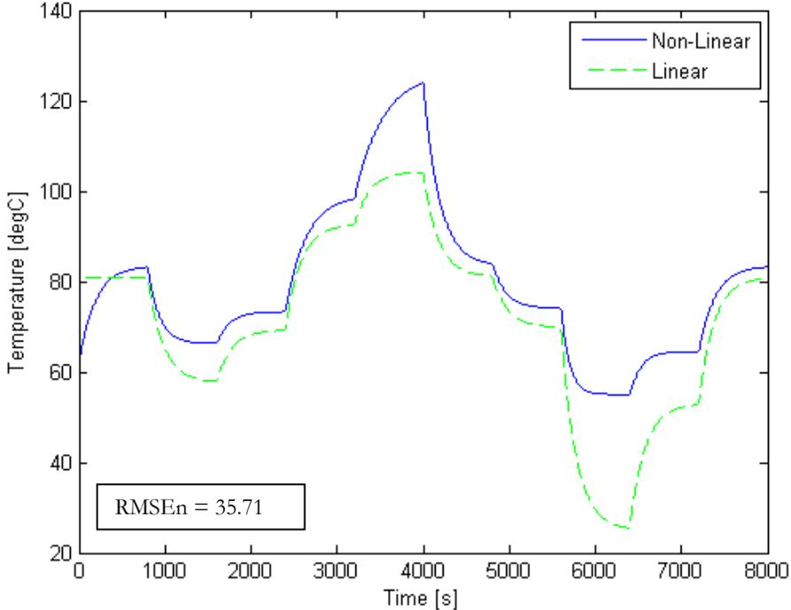
Figure 2-33 Stack Coolant Outlet Temperature at 0.2 A/cm<sup>2</sup>
