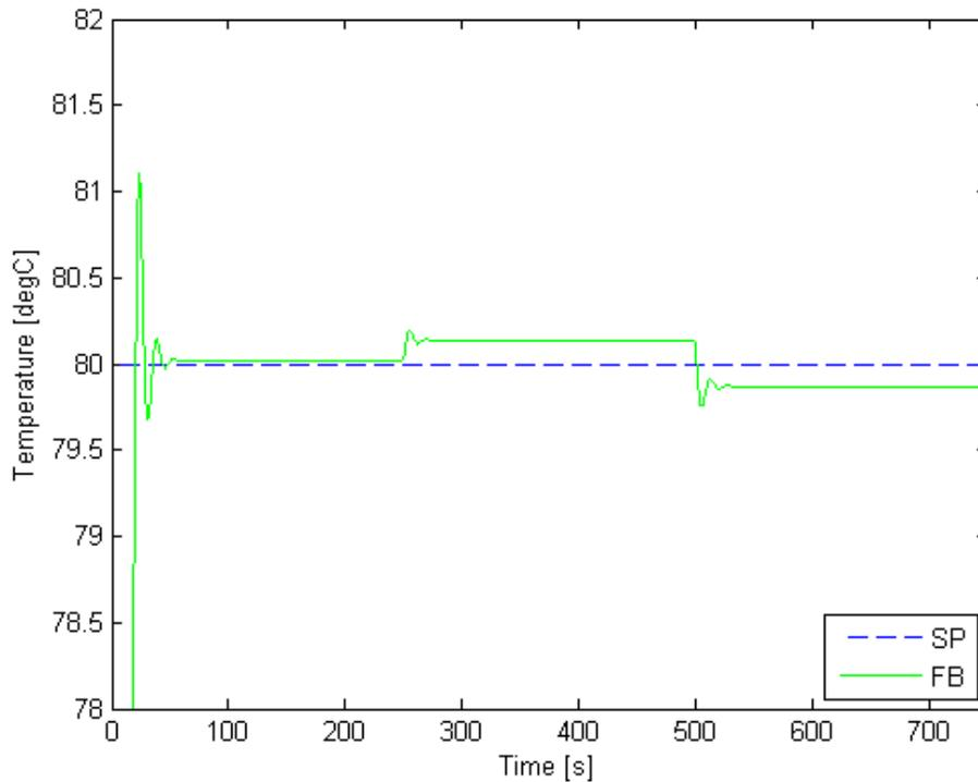
Figure 3-20 Stack Outlet Temperature: Augmented LQR Control
