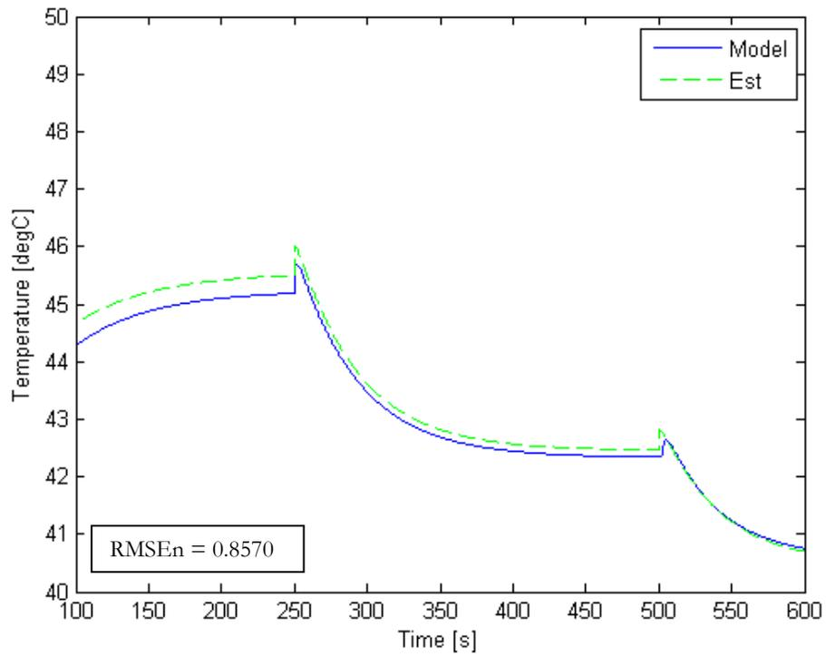
Figure 3-34 State 1: Radiator Coolant Outlet Temperature, 0.6 A/cm<sup>2</sup>
