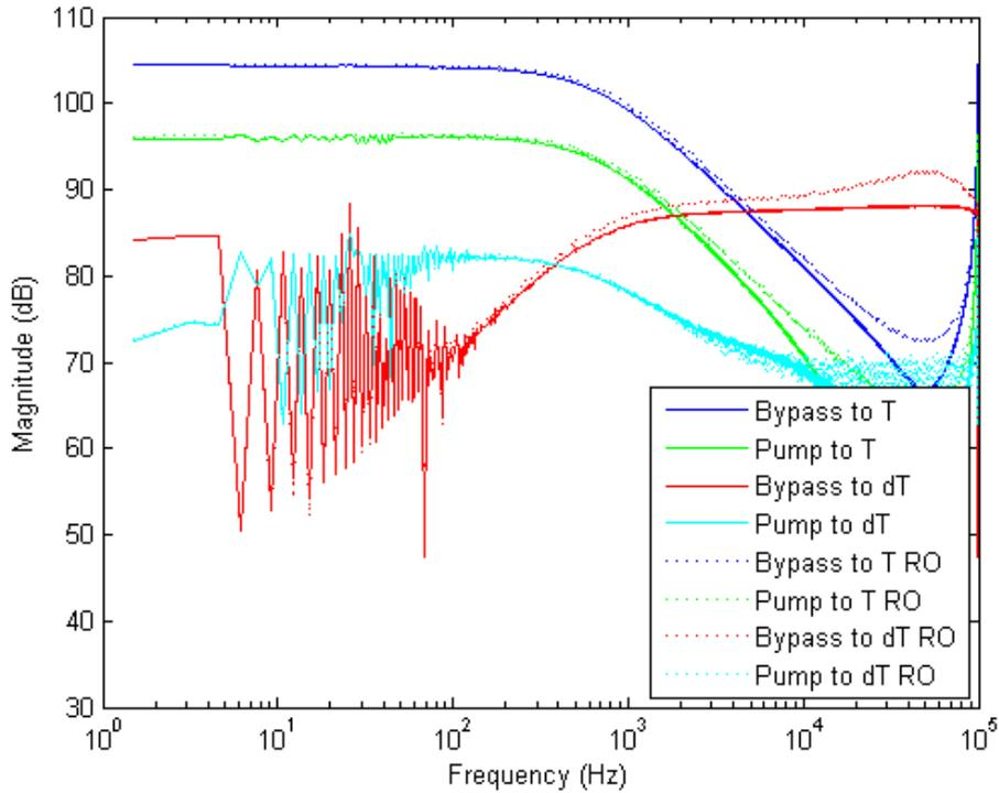
Figure 2-32 RO and Full Model FRF Comparison at 1.2 A/cm<sup>2</sup>
