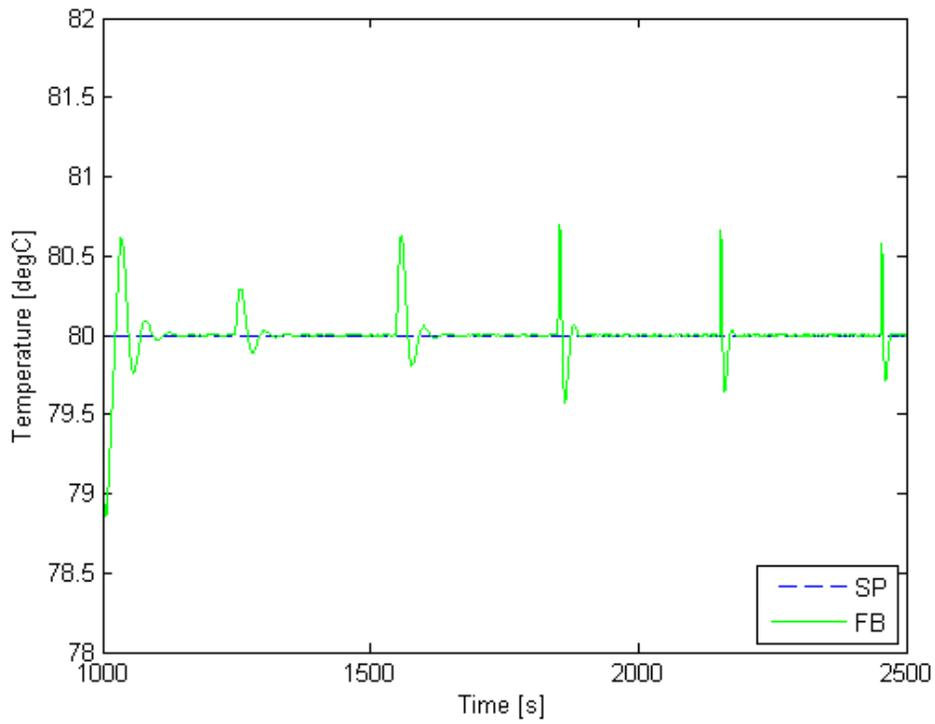
Figure 3-4 Stack Coolant Outlet Temperature: PI Control
