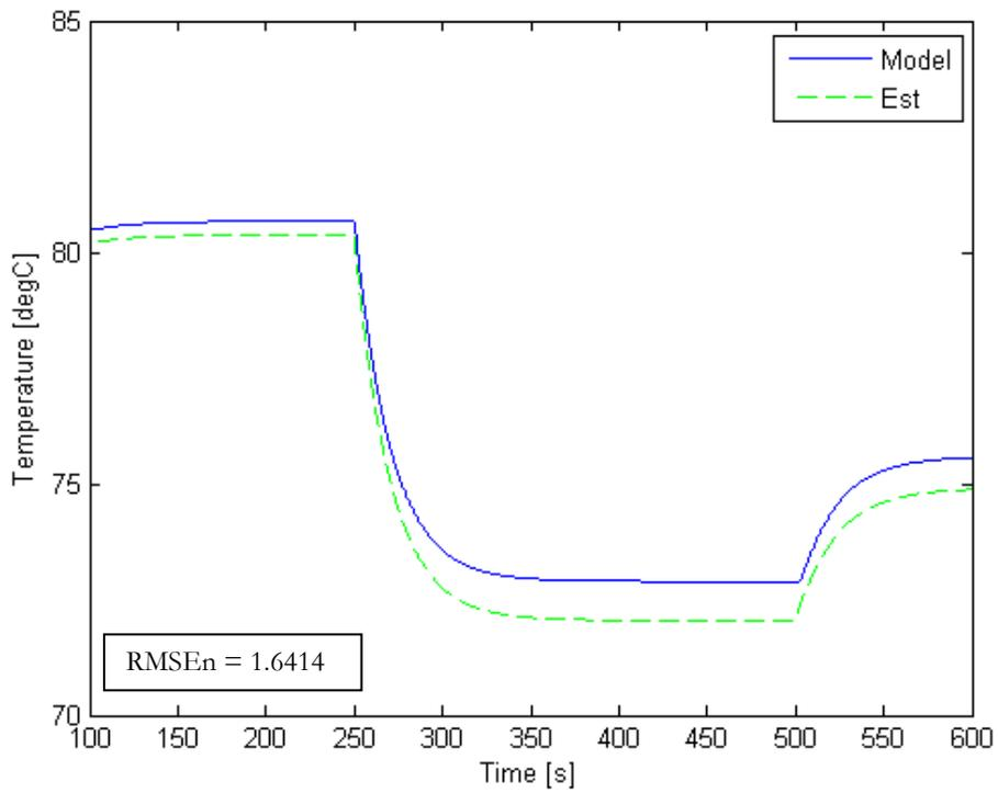
Figure 3-39 State 3: Stack Coolant Outlet Temperature, 1.2 A/cm<sup>2</sup>
