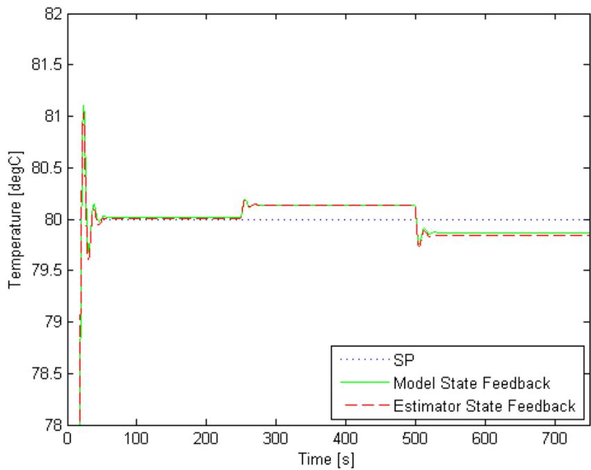
Figure 3-43 Stack Coolant Outlet Temperature: LQR Control with and without Estimator, 0.6 A/cm<sup>2</sup>
