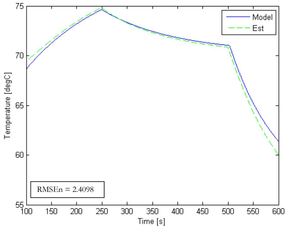
Figure 3-33 State 3: Stack Coolant Outlet Temperature, 0.2 A/cm2
