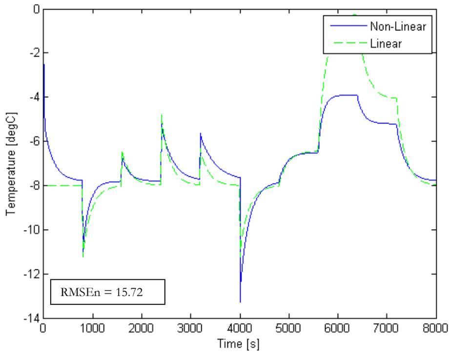
Figure 2-34 Stack Coolant delta T at 0.2 A/cm<sup>2</sup>
