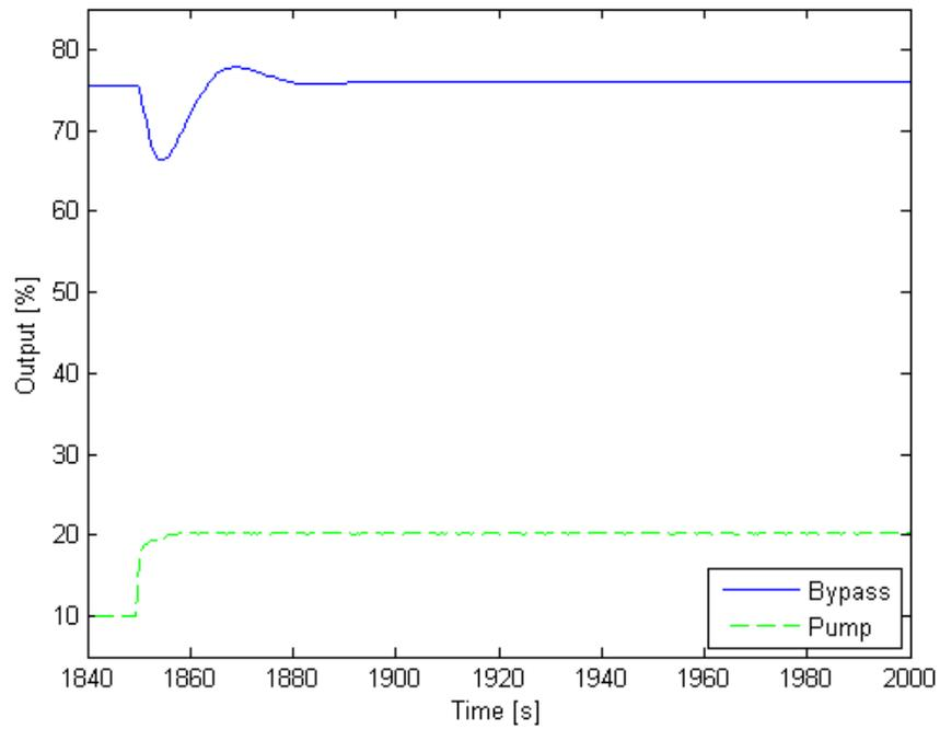
Figure 3-13 Controller Response for Step Change in Current from 0.2 A/cm<sup>2</sup> to 0.4 A/cm<sup>2</sup>: PI Control w/ sFF
