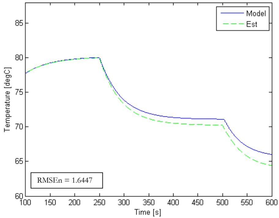
Figure 3-36 State 3: Stack Coolant Outlet Temperature, 0.6 A/cm<sup>2</sup>
