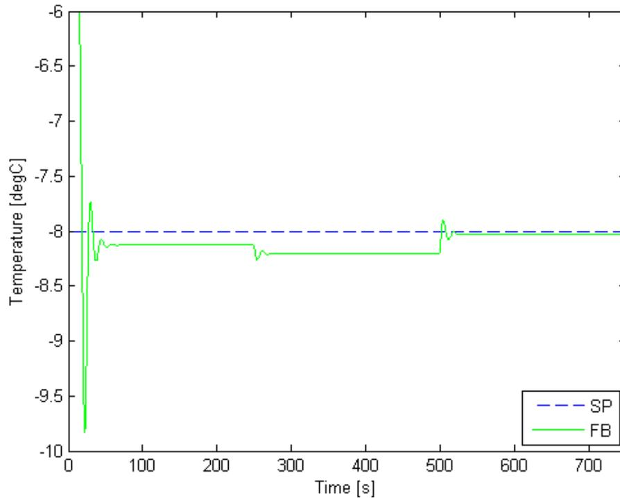
Figure 3-21 Stack  $\Delta T$ : Augmented LQR Control
