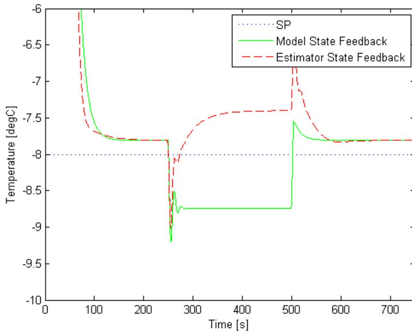
Figure 3-41 Stack Coolant  $\Delta T$ : LQR Control with and without Estimator,  $0.2 \Delta/cm^2$
