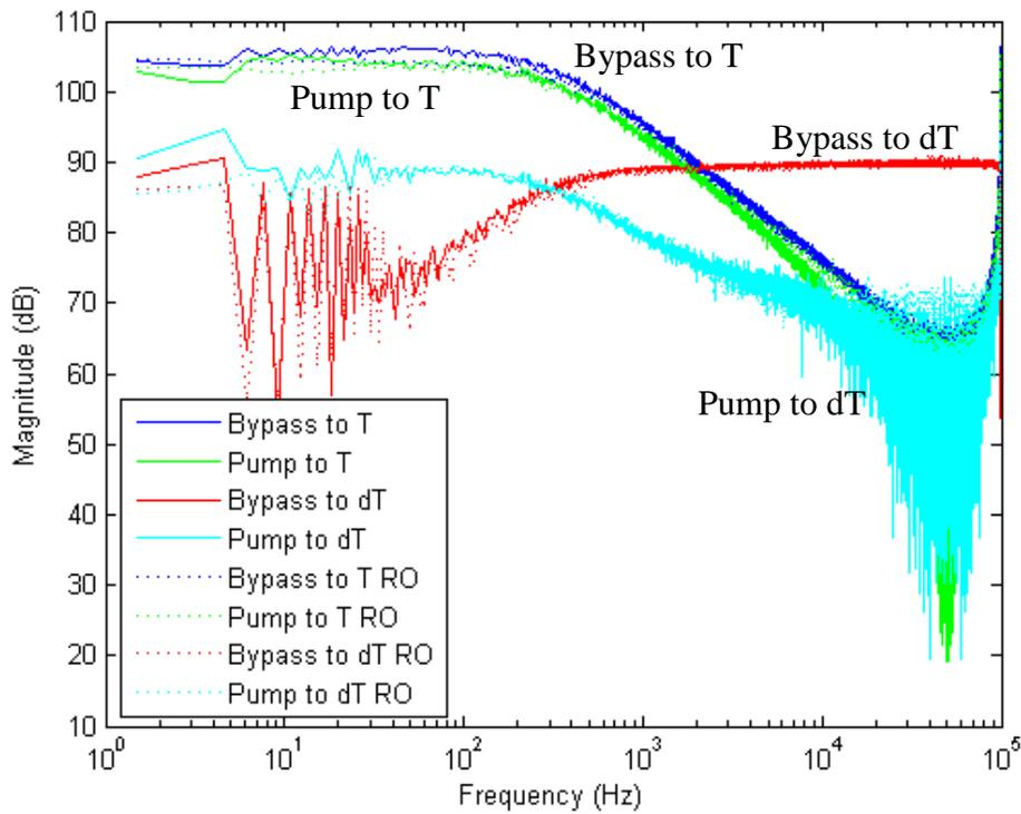
Figure 2-31 RO and Full Model FRF Comparison at 0.6 A/cm<sup>2</sup>
