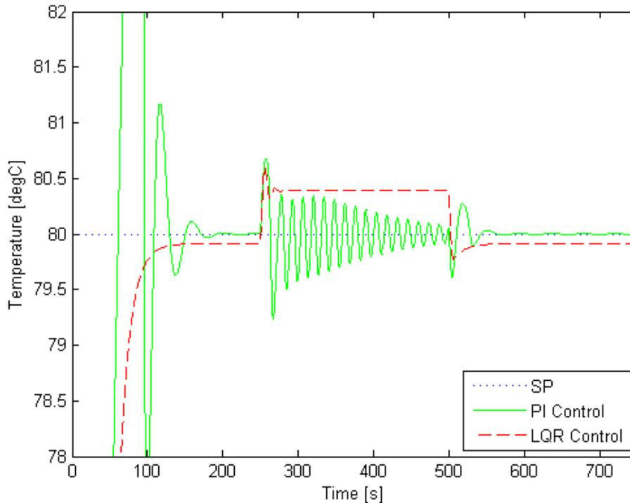
Figure 3-26 Stack Outlet Temperature Comparison
