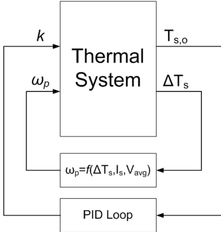
Figure 3-3 Single PI Control Loop
