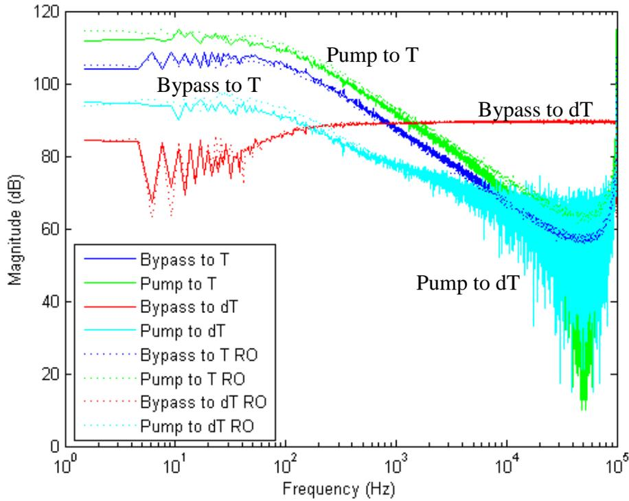
Figure 2-30 RO and Full Model FRF Comparison at 0.2 A/cm<sup>2</sup>
