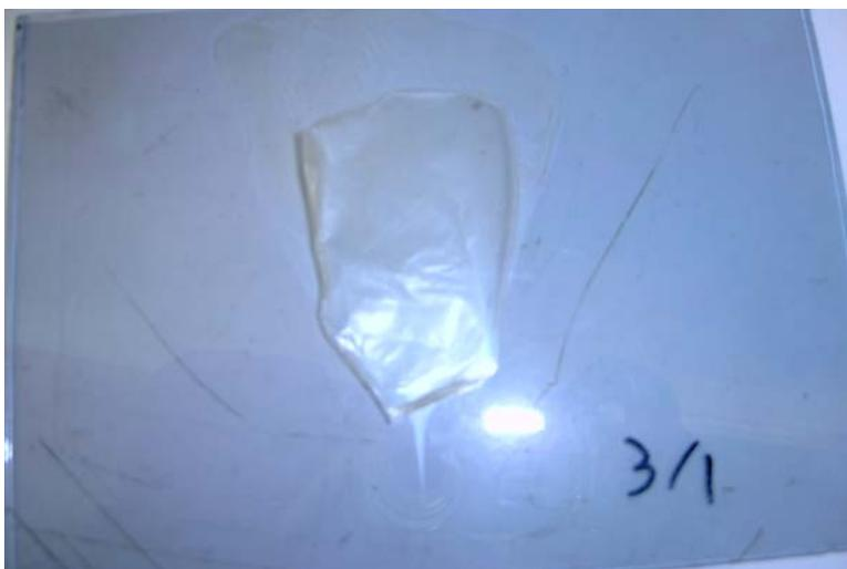
**Figure 12. Picture of composite film containing 25 volume % poly[(4(5)-VIm/VIm<sup>+</sup> TFSI)(1/0.5)<sub>M</sub>], annealed at 200°C**
