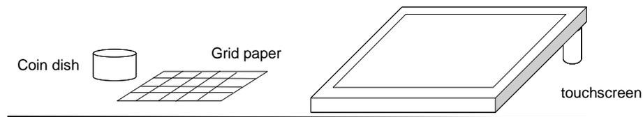
**Figure 3: Touchscreen test set-up**
