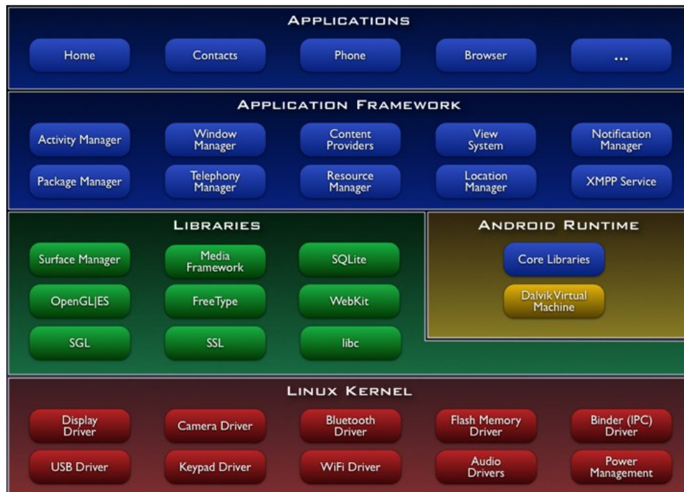
Figure 2.4: Android Operating System Architecture (Source: Google)
