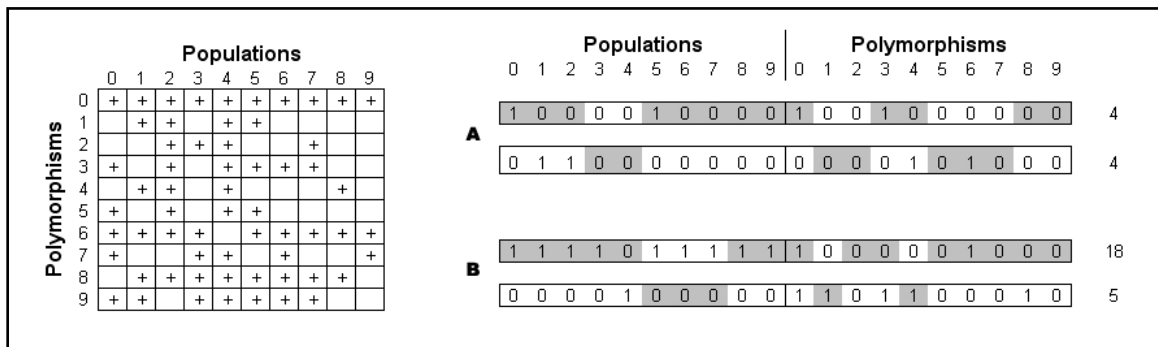
Figure 2.8: A hypothetical data matrix, and the mating of two set of parent chromosomes. A and B represents two sets of parents chromosomes ready to be crossed over at 6 random crossover points.
