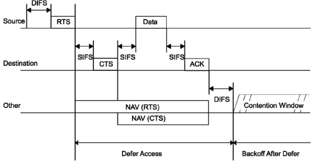
Fig. 14. Operation of 802.11 DCF (RTS/CTS access method) [6]
