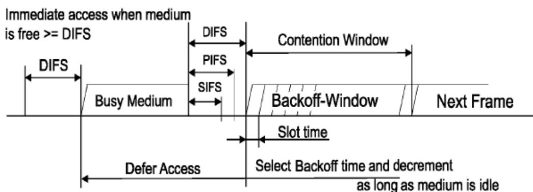
Fig. 13. Operation of 802.11 DCF (Basic access method) [6]
