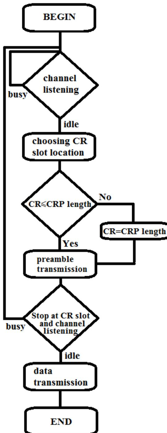
Fig. 3. Operation of an end device using BCSMA/CA
