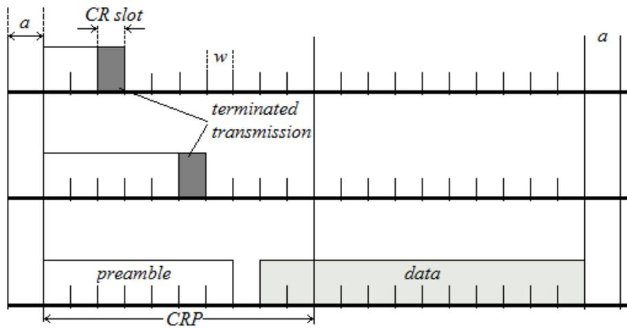
Fig. 1. Successful collision resolving
