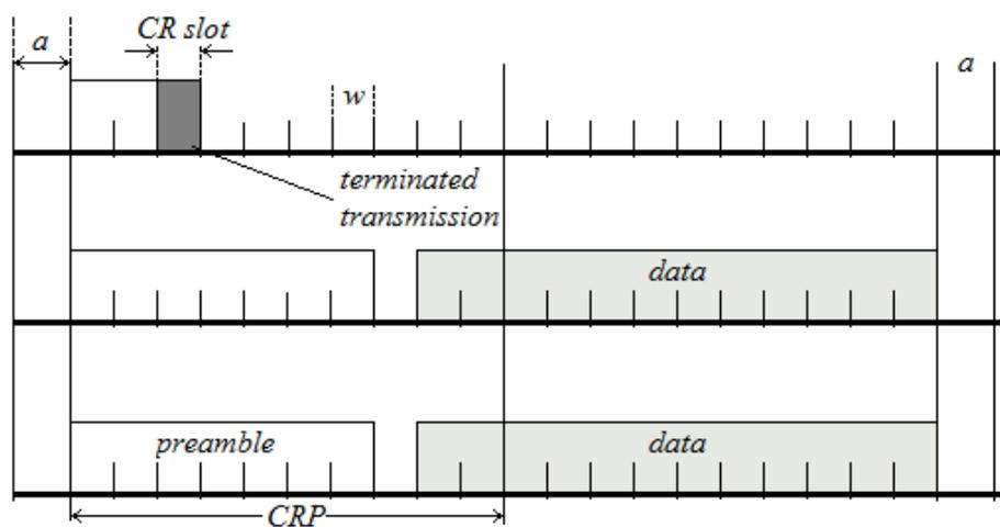
Fig. 2. Failure of collision resolving
