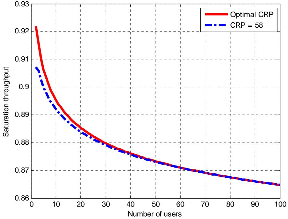
Fig. 8. Saturation throughput for optimal and sub-optimal CRP values
