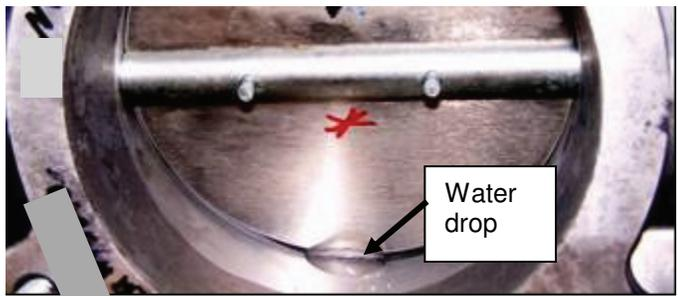
**Figure 3. Typical location and appearance of ice from laboratory test No 2.**
