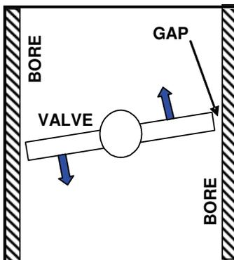
**Figure 1. Simple diagram of a throttle valve**
