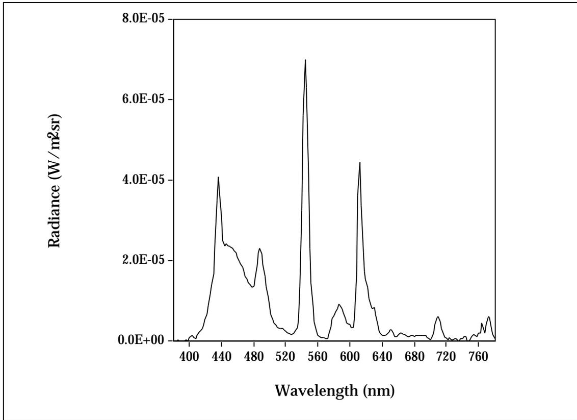
Figure 2. Spectral radiance distribution of the monitor black.
