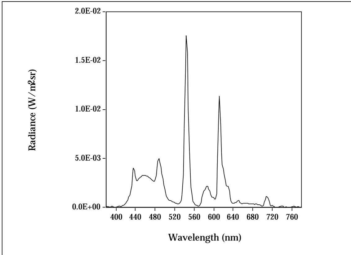
Figure 1. Spectral radiance distribution of the monitor white.
