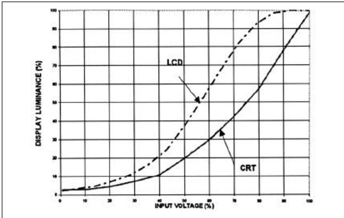
Figure 8. Typical electro-optical response functions for a CRT and LCD (from Glasser<sup>2</sup>).
