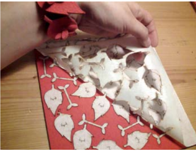
Laser cut prototype of the students' design manufactured by Ponoko.com
