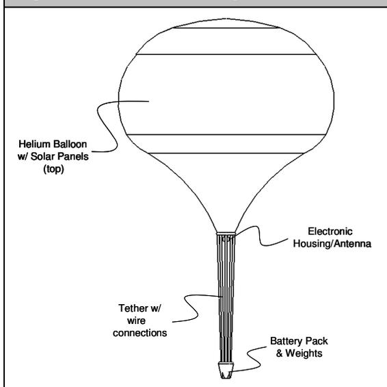
Through these meetings, another design was formulated that had a strong correlation with the structure and basic concept of a hot air balloon. This idea would allow a smooth/controlled landing of the network. In other words, the network would be attached at the base of the helium filled balloon and have solar collecting panels at the top of the balloon. See Figure 4 for more details.
