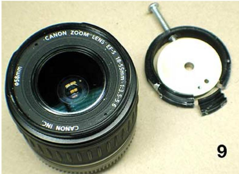
Finally, as shown in 7, I dropped the piece of the split-ring that I had cut out of the larger ring into the open space opposite the threaded bolt.
