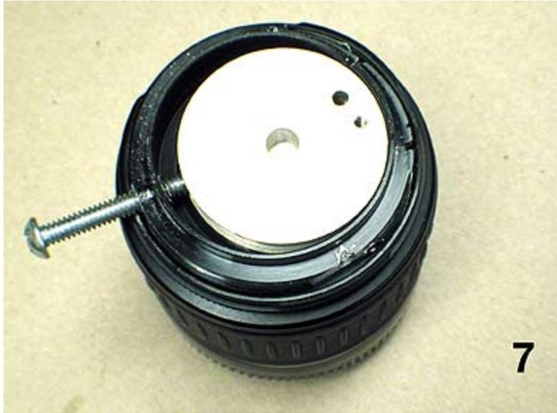
Into the tapped hole I screwed a bolt. Then I found a metal disc that was somewhat smaller than the diameter of the inside of the metal ring out of which I had cut a section. See figure 3.
