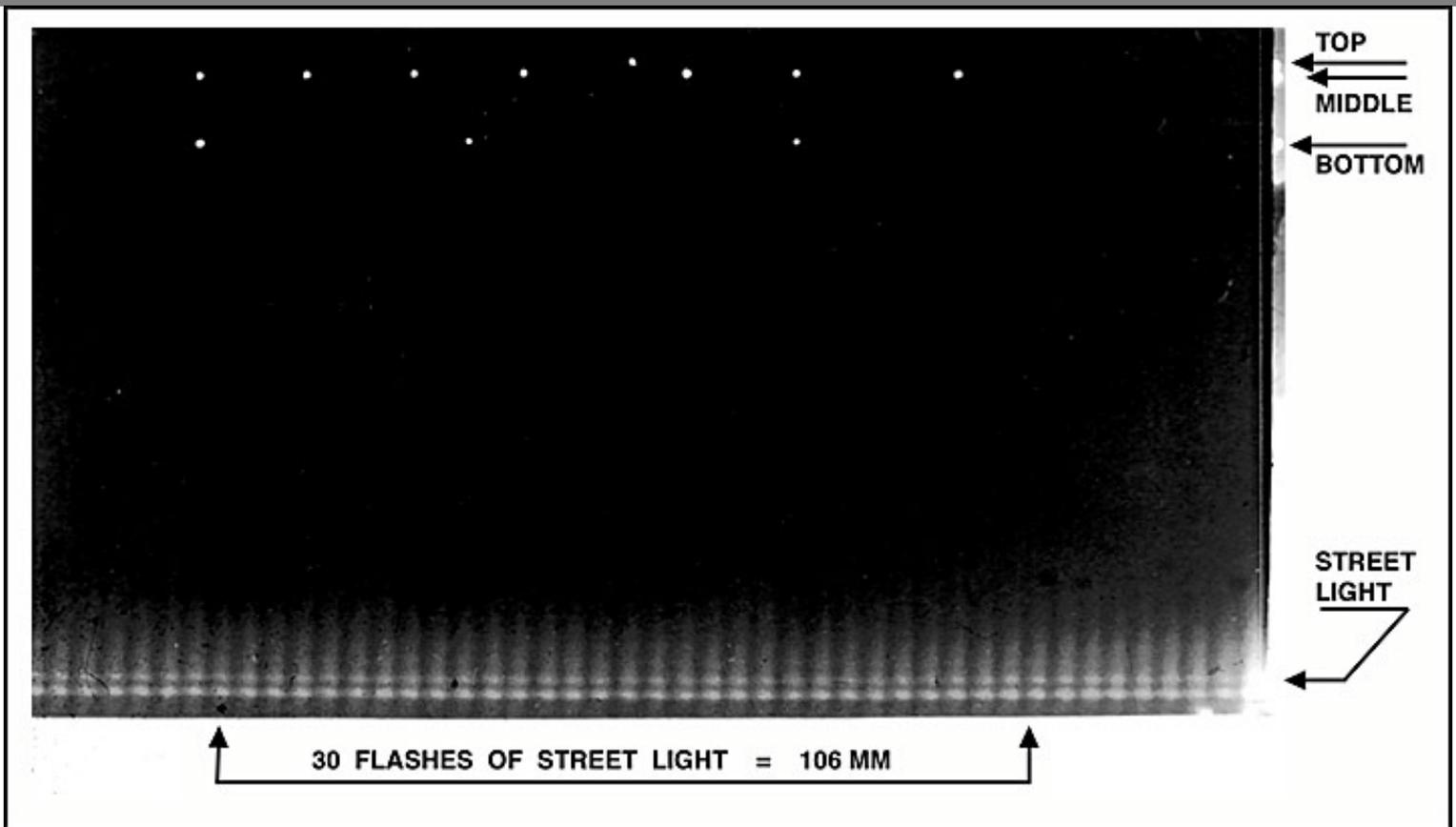
Sample print taken with the streak camera showing dots corresponding to the strobe flashes and a regular pattern of dark and light bands created by the sodium vapor street lamp.
