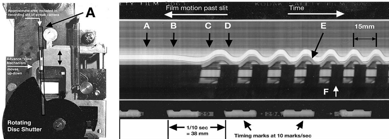
Analyzing the claw/shutter movement in a motion picture camera (note that it takes the camera about four to five cycles to settle on a steady pattern as the motor picks up speed). A—Camera stationary. B—Movement starts. C—Claw moves up during first exposure. D—Claw moves down bringing fresh film to gate during shutter's closed period. E—Up-down motion of claw mechanism. F—Rotary sector shutter.
