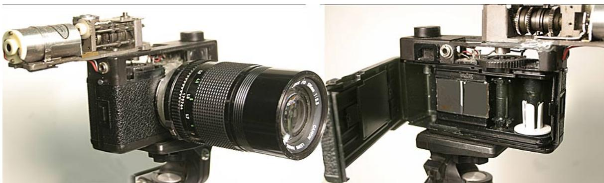
Left: Front view of the modified camera, with stripped motor attached to the top to power the film transport. Right: Open back view of the camera, showing the 1mm wide slit in the mask in the focal gate.
