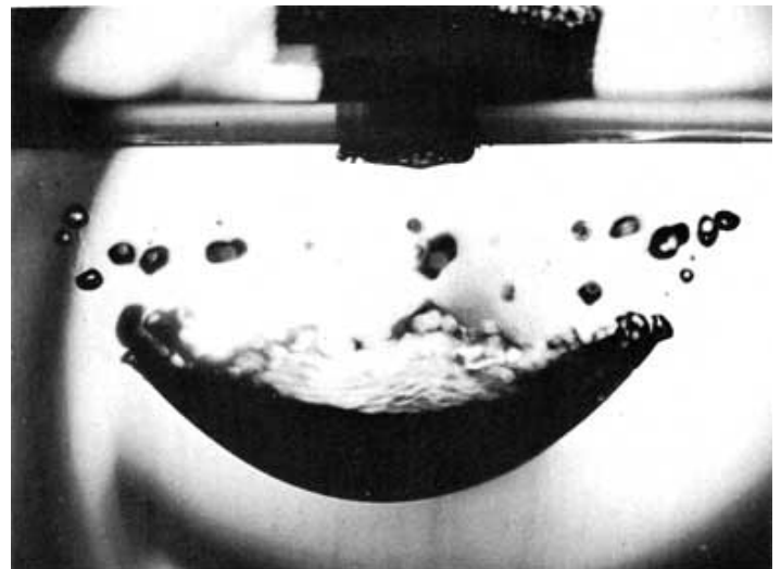
Figure 4. Boule burst after 70% collapse by Strobflash lighting. Note that shroud was moving too fast for the duration of this flash. Detached bubbles remaining from shroud float towards surface.
