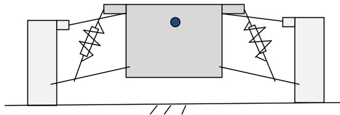
Figure 7 Schematic of the Tundra Front Suspension
