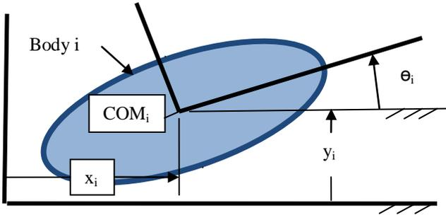
Figure 2 Coordinates Describing the Position of a Planar Body
