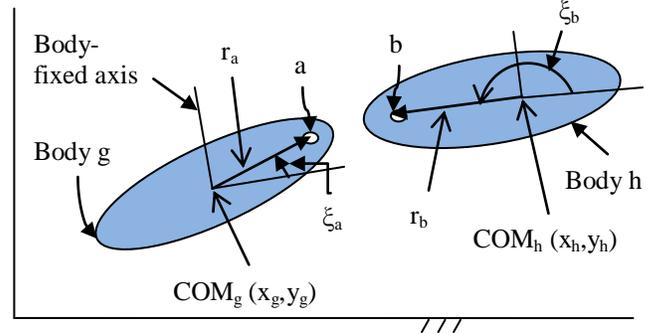
Figure 3 Virtually Separated Revolute Joint
