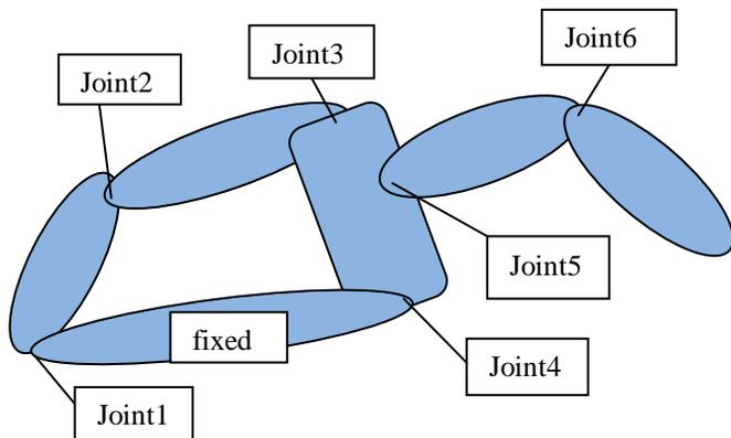
Figure 1 Representative Combined Closed and Open Loop Mechanism
