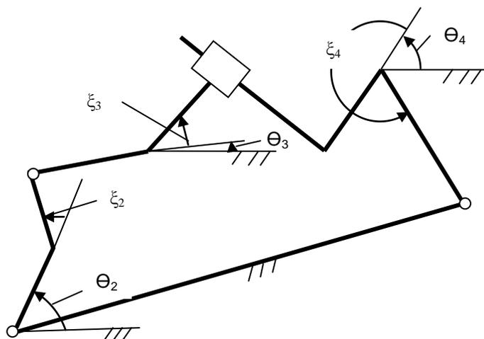
Figure 10 Generalized Inverted Slider Crank Mechanism
