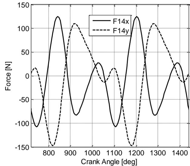
Figure 9 Example Planar Fourbar Follower Ground Pin Reaction Forces vs.  $\theta_2$  [deg]
