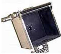
It was made with a home-built moving slit type matte box shown in the illustrations below. The device reminds one of an oversized lens shade and consists of a 12 inch cube made out of plywood that has an open front and on the back wall it has a hole through which the camera lens looks into the box.
