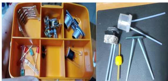
Figure 3. Real circuit elements (left) and their models for blind/low-vision learners (right)
